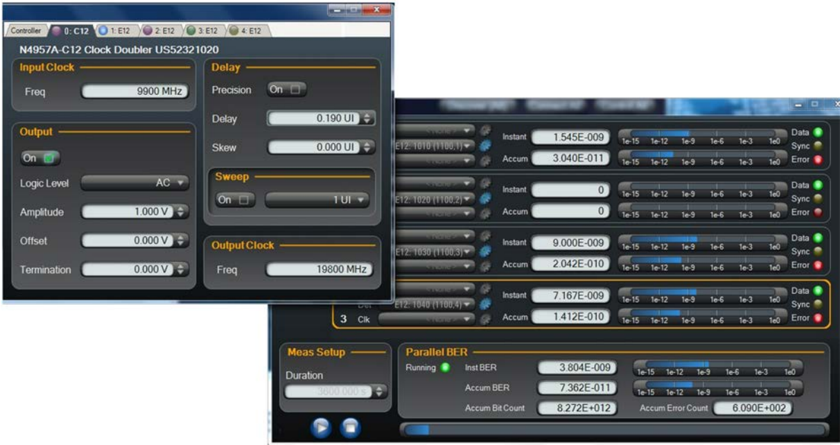
Figure 12. Increase delay until errors occur
